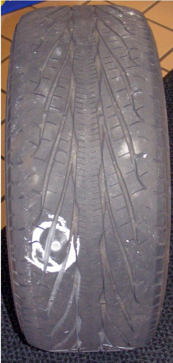
Even steel-belted radials get punctures. Some puncturing objects are small, some are quite large. This is a tire from my Aurora which acquired a nail. Two photos on the opposite panel show a close-up of the nail head and the interior view of the nail. It wasn't even a whole nail—just a stub of nail. How embarrassing! 😊
