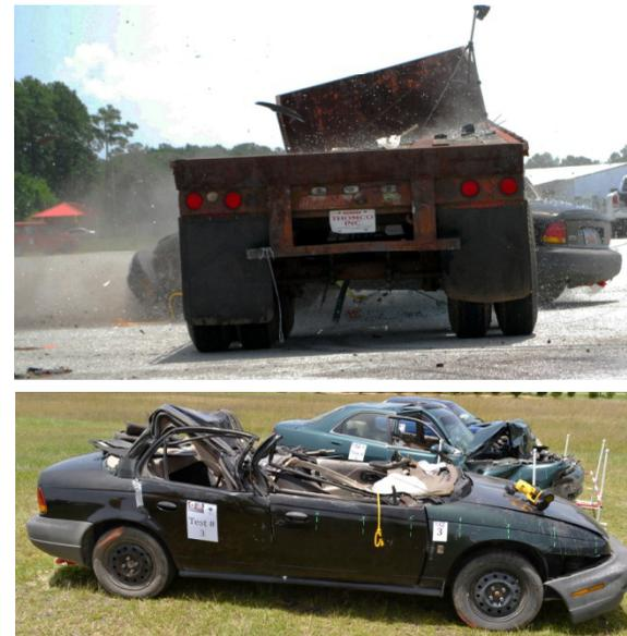
The photo immediately to the left of this text shows the collision in its final stages. This trailer was not connected to a truck tractor, so it twisted as a result of the forces being applied to the underside. And you thought these semi-trailers were rigid! After impact, the trailer returned to its normal shape, with no structural damage as a result of the under-ride.
