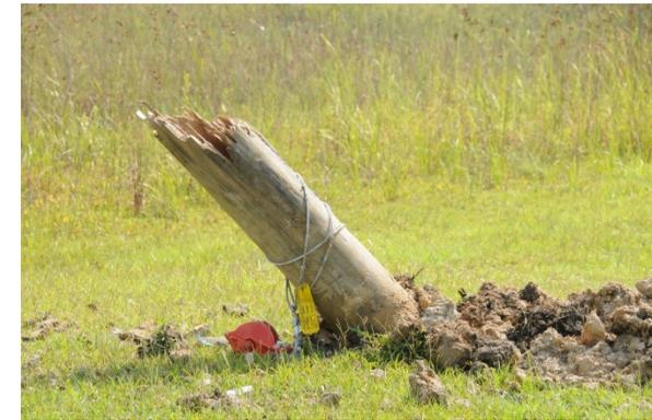
As you can see in this photo sequence, the Saturn was completely airborne as it rode up the stub of the broken pole. The separated upper section of the pole struck the top of the Saturn as it traveled to its final position. The impact speed of the Saturn was approximately 41 mph.
