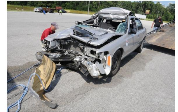
data in the PCM. The tractor-trailer was moved 21 inches by this second impact, indicating a delta-v for that truck of 4.5 mph. Interestingly, the speedometer of the second Ford involved in the rear underride testing was found stuck at 52 mph after the crash, although its impact speed of 38 mph was well-documented and verified. Sometimes a stuck speedometer or tachometer needle means something, sometimes it doesn't.
