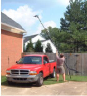
This photograph was taken with a digital camera to show the technique involved in taking an overhead shot of a vehicle. The idea, of course, is to provide a bird's-eye view of a collision-damaged vehicle to help graphically portray the damages, hopefully to clearly demonstrate the principal direction of force (PDOF), an important parameter in most accident reconstructions. This setup uses a light stand, a 35 mm SLR camera with motor winder, and remote shutter firing.
