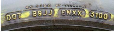
The 3100 at the end of the code indicates that this tire was made in the 31<sup>st</sup> week of 2000. Tires manufactured in the previous century had only a three-digit final code. A serial number is not unique to each tire; it is unique to each tire made on the same assembly line at the same plant in the same week.
