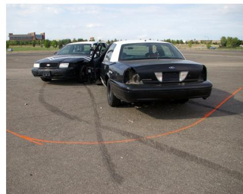
This shows the result of the first staged collision, which involved two geriatric police cruisers. It fortunately happened to be a perfect example of a center-of-mass-to-center-of-mass collision, easy to evaluate but difficult to stage. This collision occurred at relatively low and documented speeds and was used to demonstrate the validity of several aspects of accident reconstruction, including the reduction of effective drag factor for offset motion.
